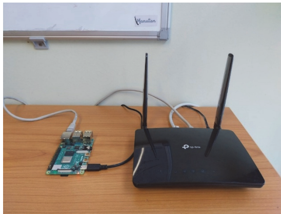
Figure 4: Raspberry Pi unit connected to a router, serving as a central hub for smart home automation and energy monitoring tasks.
